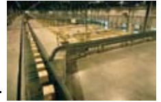
A first in U.S. elections we use moving conveyors - similar to those used in freight sorting facilities - to sort all election supplies on Election Night. This reduces labor costs and shortens the time needed to certify election results.
